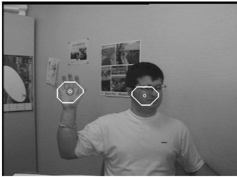
Figure 2. Example of blobs on the face and the hand represented by polygons
